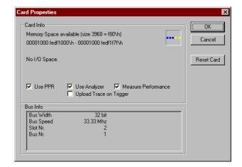
This dialog box contains information both on the testcard and on the PCI bus it is plugged into. For the *Card Info* this includes the address range of the memory space and the I/O space together with the four check boxes:
