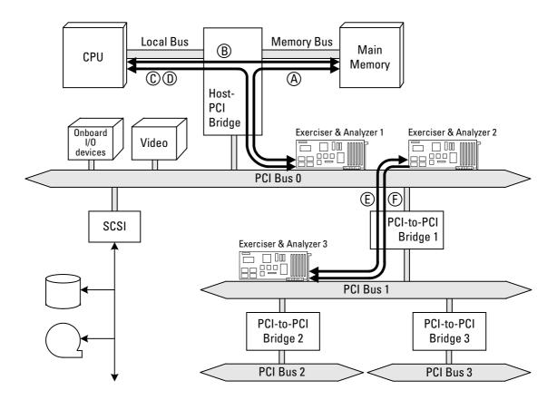
Additionally, the System Validation Package also provides tests that cause the testcard to generate traffic to itself via the PCI bus to increase the bus load, and tests that analyze the performance of the bus.
