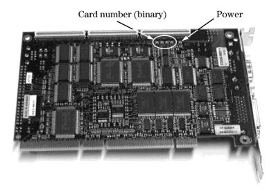
**Power LED** The LED at the rear end of the row is slightly further separated than the others. It is always lit, when the card is powered.
